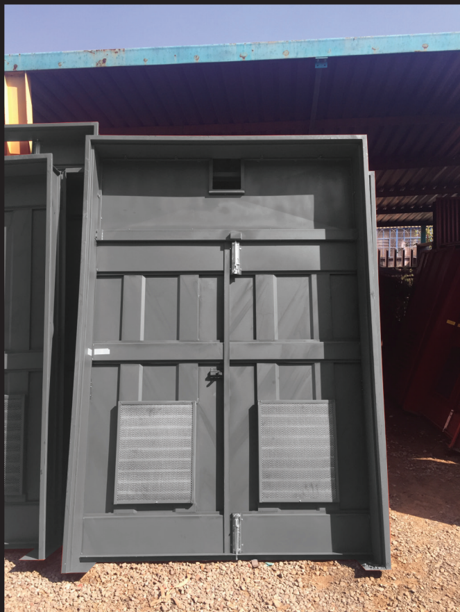
Fanlight removable panel & crawl beam cut out
