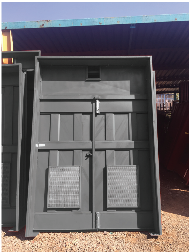
Fanlight removable panel & crawl beam cut out
