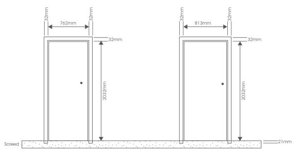
Widths are into rebate of frames. Heights are from finished floor to head rebate.
