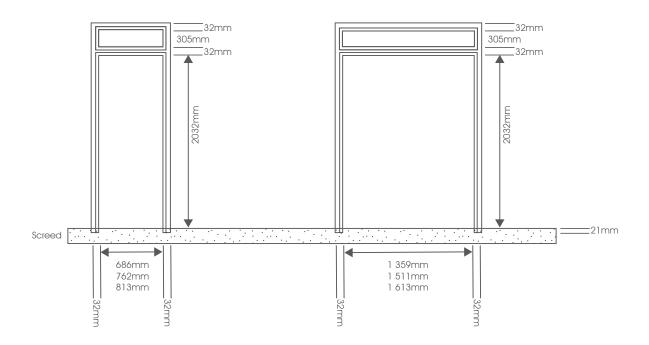
Note: Non-screeded Door Frames are 2064mm in overall height, which is 21mm shorter in length than screeded frames
