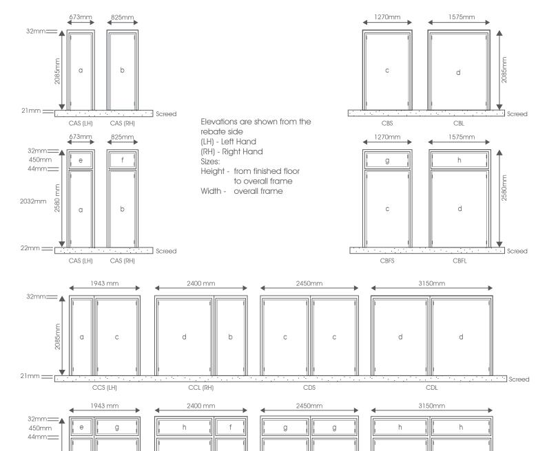
Widths between rebates and heights from finished floor to rebate at Head are as follows:
