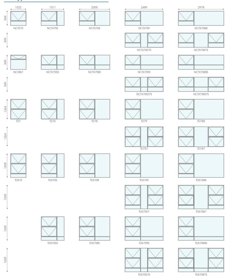
$<sup>^{\</sup>star}\text{Glass}$  not included with frames - shown for illustration only All F7 Windows will have a width shortage of 25mm in comparison to your FX7 Window.
