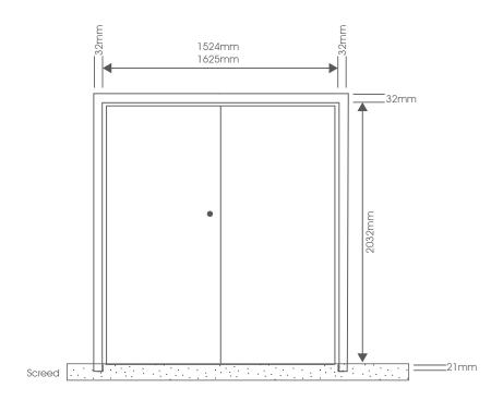
Widths are into rebate of frames. Heights are from finished floor to head rebate.
