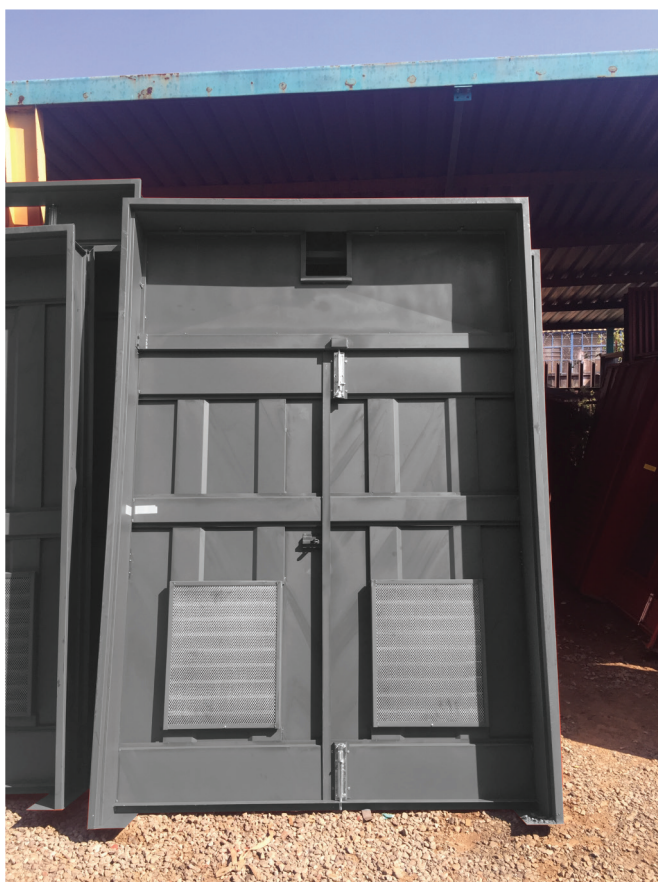
Fanlight removable panel & crawl beam cut out
